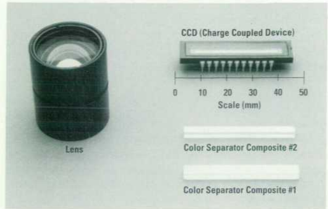
Fig. 4. Lens, CCD detector, and color separator composites.
