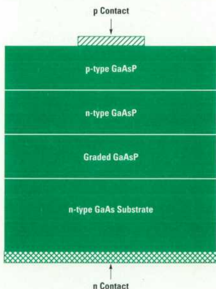
Fig. 1. GaAsP standard red homojunction LED.
